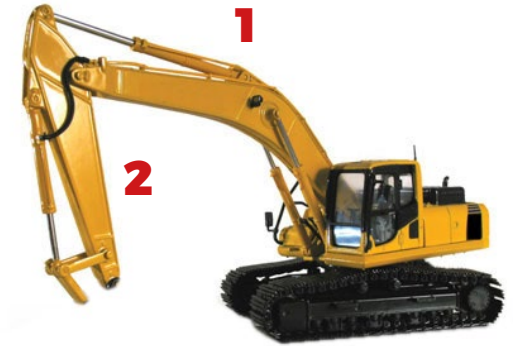
Two-Piece Boom (Increases rigidity and reduces cost compared to a 3 piece boom)
