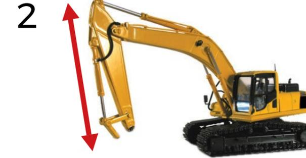
Short Dipper Boom & Large dia. Pivot Pins
